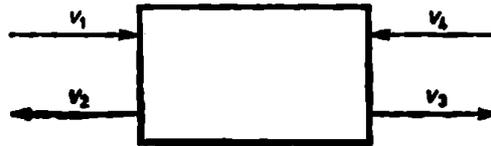
where  $v_1$  and  $v_4$  are the incident waves and  $v_2$  and  $v_3$  are the reflected waves. These waves are related by the following transformation
